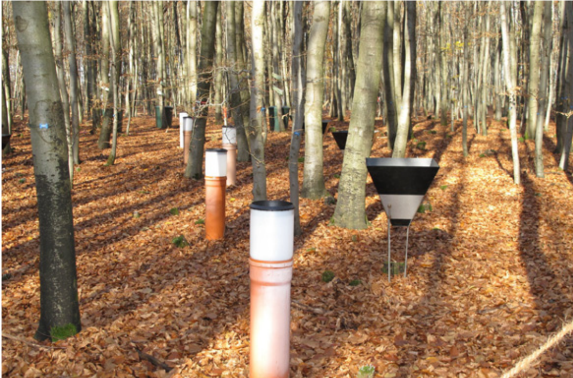
Experimental site: measurement of precipitation (© ForeStClim)
