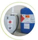
step 4 Titrate oil and add Methanol and Methylate to pre-mix container
