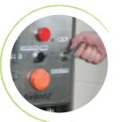
• step 3 When at 60°C turn valve to Oil Fill
